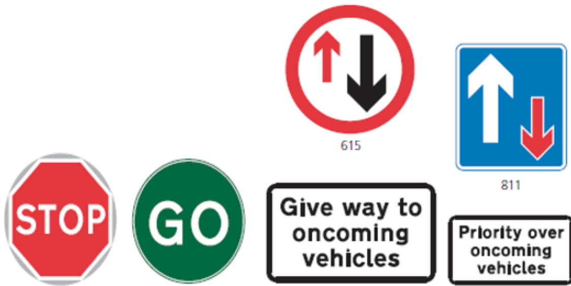
Figure 1.5: Manually operated stop/go signs and priority signs
